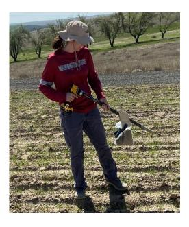
Figure 11. Dr. Olivia Landau collecting soil samples using the customized soil sampler. The sampler was designed by Dr. Stuart Wuest (USDA-ARS, Pendleton, OR). In summary, the sampler is a drill bit auger covered by a metal sheath. The metal sheath has an opening that allows the collected soil to be funneled into a bag as the researcher is sampling through the field. The diameter of the auger is 1.0"
