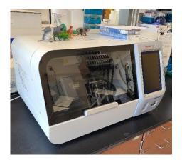
Figure 14. The Thermo Scientific KingFisher Apex, a high-throughput extraction system capable of processing 96 samples simultaneously. This instrument supports DNA, RNA, and protein extraction, with specialized kits for plant tissue and soil samples for microbiome analysis.
