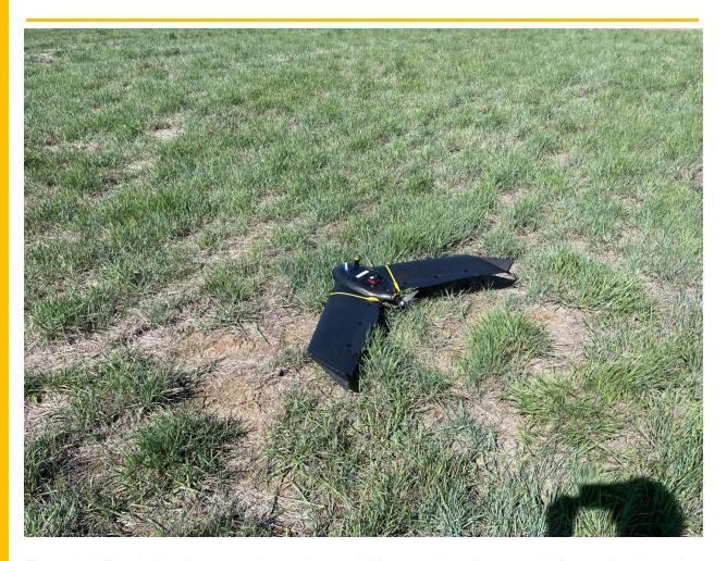
Figure 39. Fixed wing drone used to collect aerial imagery in order to track the spatial dynamics of weed populations. April 2025. Whitman County, WA.
