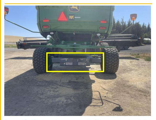
Figure 38. A Seed Terminator unit mounted on a combine for harvest weed seed control. July 2023. Whitman County, WA.
